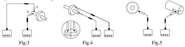
For measuring the axis displacement the transducer is placed parallel to the axis at the flange of the shaft and/or parallel to the testing clamp plane (*Fig. 4*).
